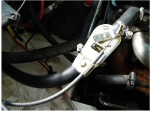
hot, it slides right on, but be careful, I ended up donating some skin off a knuckle. It slid onto the plastic valve much easier. Don't forget the clamps, and put the whole assembly together. Bob's rule is to never put the screw
