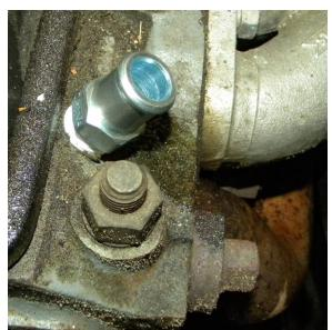
part. The piece of 1/2" goes from the valve to the Firewall port. This means you need to force a piece of 1/2" hose onto a 5/8" port on the valve. Attach this hose to the valve first. I clamped the valve in a vise, lubed the hose with WD40, and heated the hose with a heat gun. Once it's
