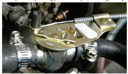
the wire in place, I added a #10 washer, and a short length of Vacuum hose. This setup is actually easier to operate, and at worst, if it fails, it will just drip rather than emptying out your cooling system. For what it's worth, I put the same setup in my TR3B, by adding a second choke cable to control the valve. For those of you unfamiliar with the TR3, there was a manual valve in the same location, so you needed to lift the hood to adjust the heat. Not my idea of fun on a cold day.
