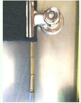
Brass tube to distribute the water. Below, water supply tubing.
