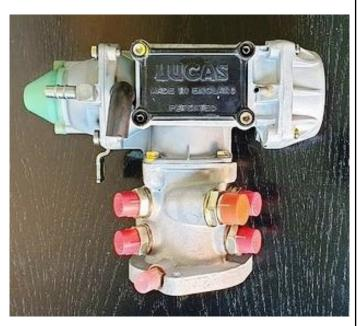
Clearly if you lived at these altitudes (where RMTC lives) the car would be no good to you at all. This was Triumphs mechanical solution. The capsule on the bottom detects atmospheric pressure and compensates by reacting against the metering spring pressure to lean off the mixture proportional to altitude. Simple but effective. I dare say that if PI had continued, all metering units would have morphed into a version of this.
