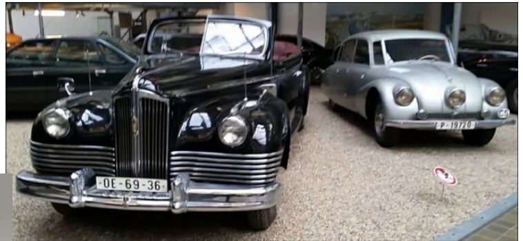
1952 Zis parade car, built in Moscow, a clone of a 1937 Packard.. Also, a 1937 Tatra, with a 3000 cc air-cooled rear engine V8.
