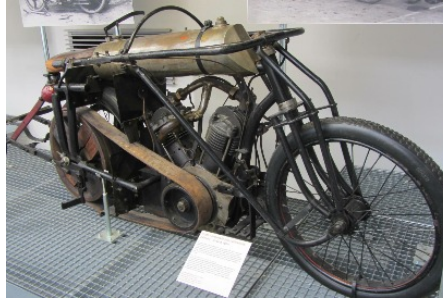
1910 Kolem windbraker for bicycle record attempt, it has no gearbox.
