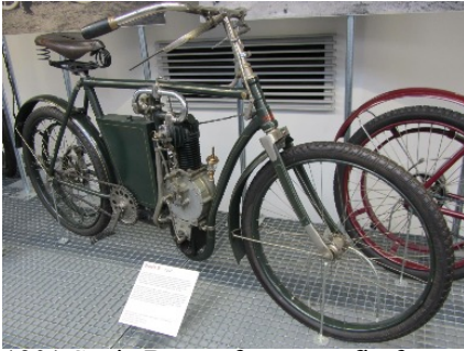
1901 Savia B, note frame config for engine
