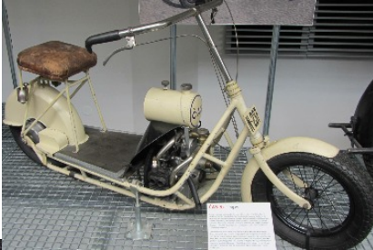
1901 Savia B, note frame config for engine
