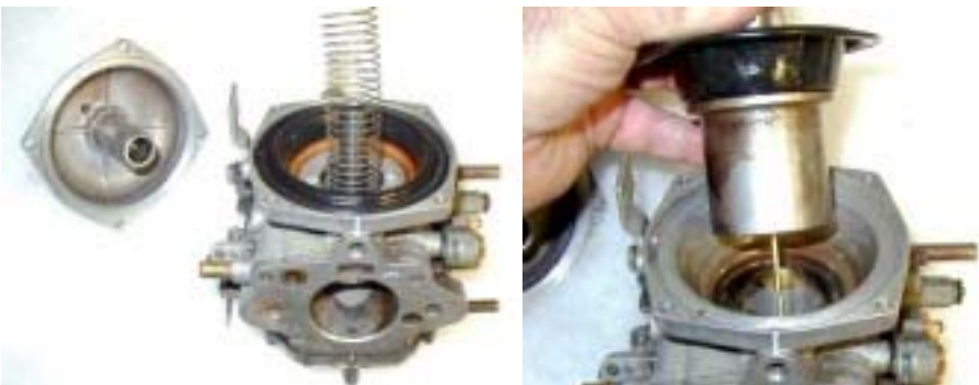
The top cover is removed first using a Posidrive screwdriver.
