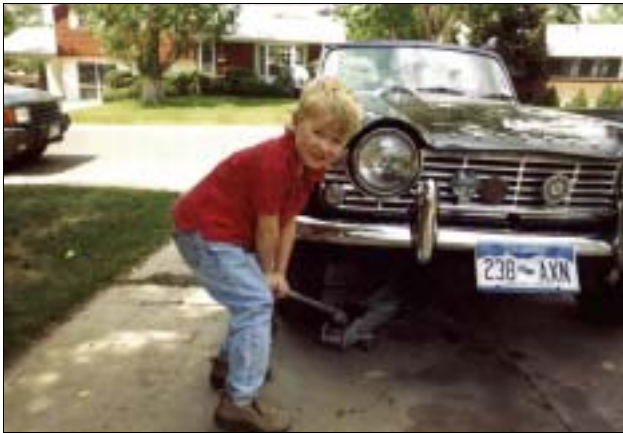
Ben Newell, Steven & Pam's son demonstrates proper front jacking location for a TR4.
